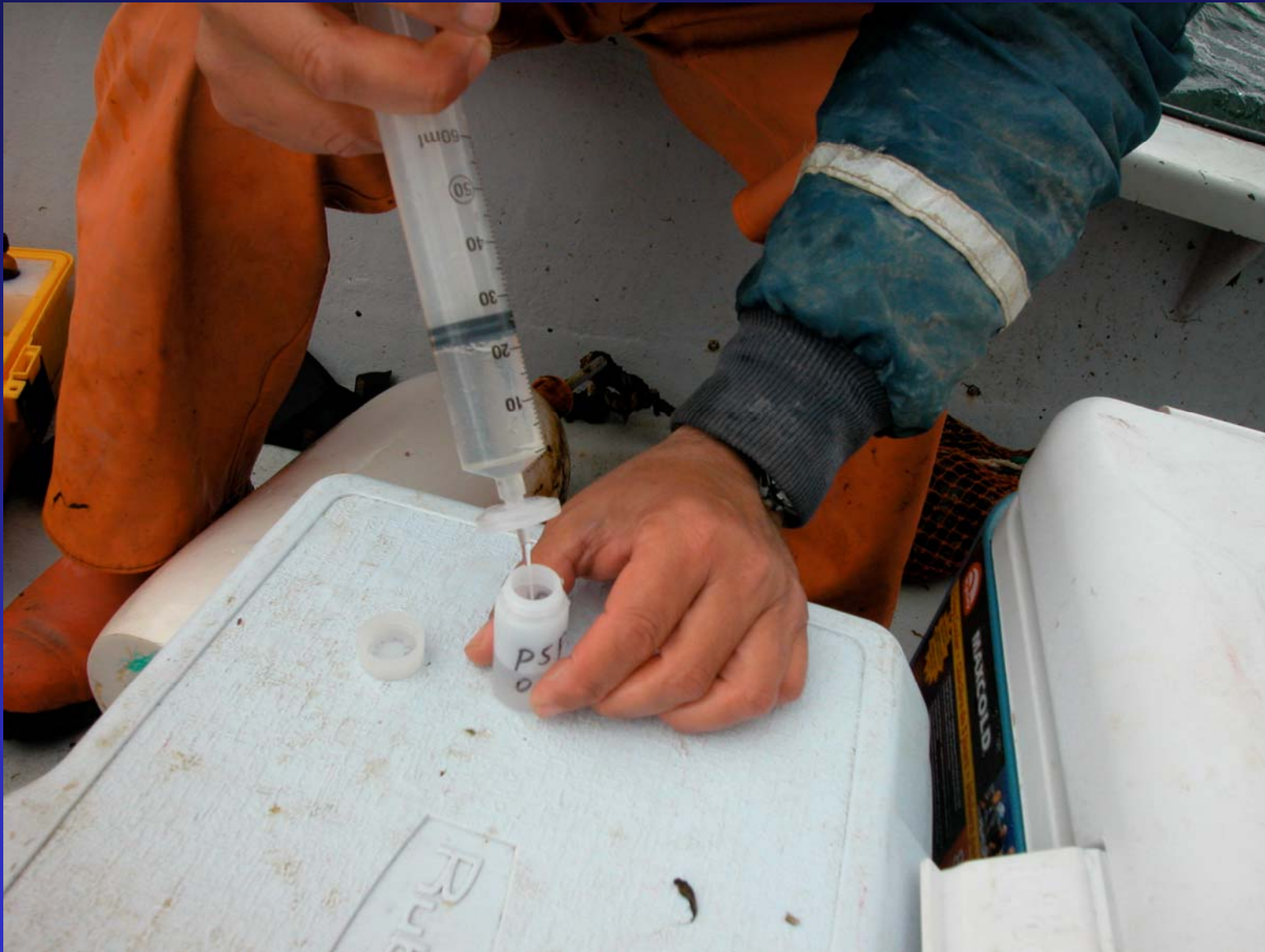
Nutrient samples are filtered into sample container, then placed on ice.
