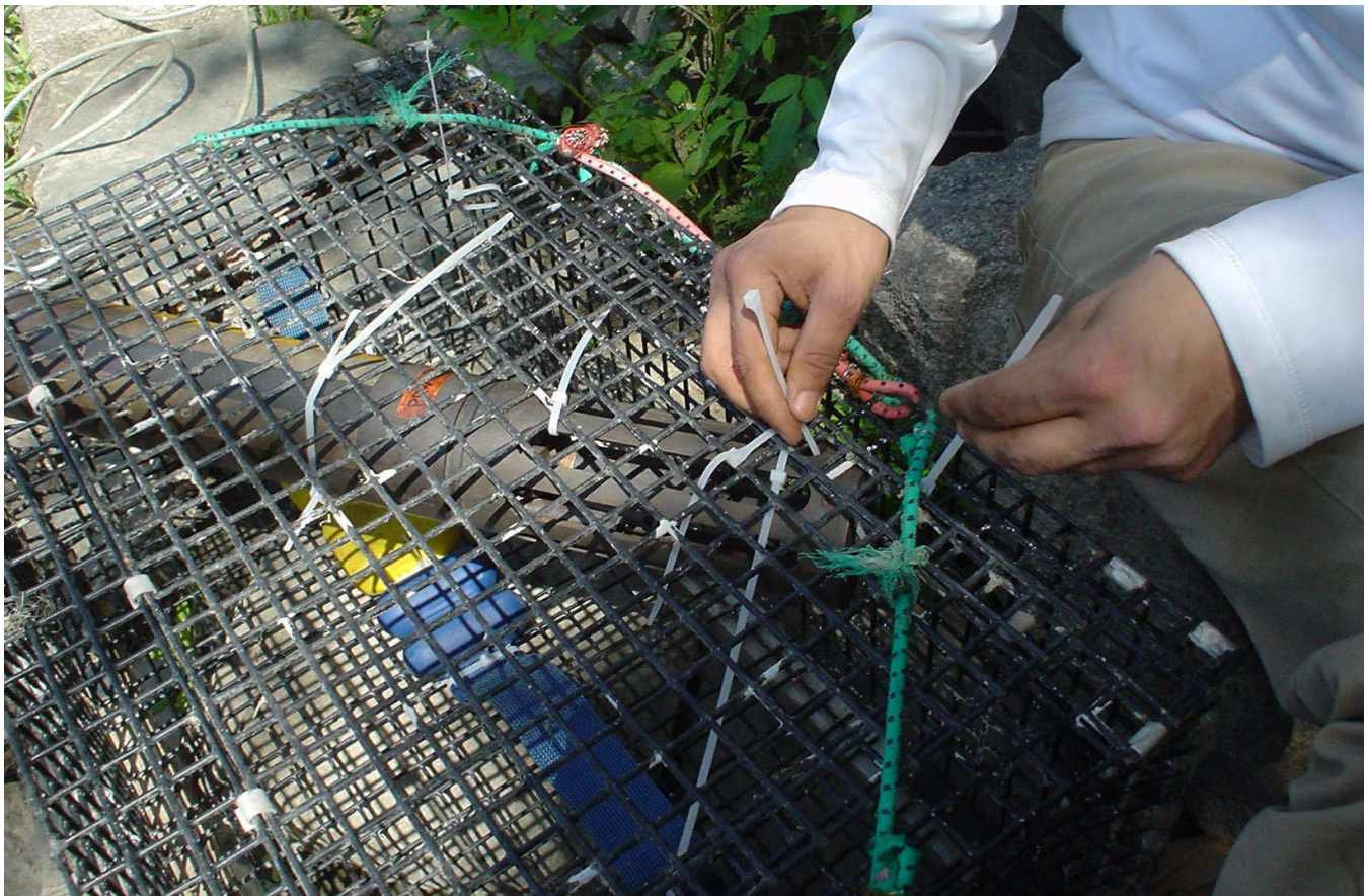
Figure 3: Close up of datasonde deployment method, with diving weights attached to bottom of cage.
