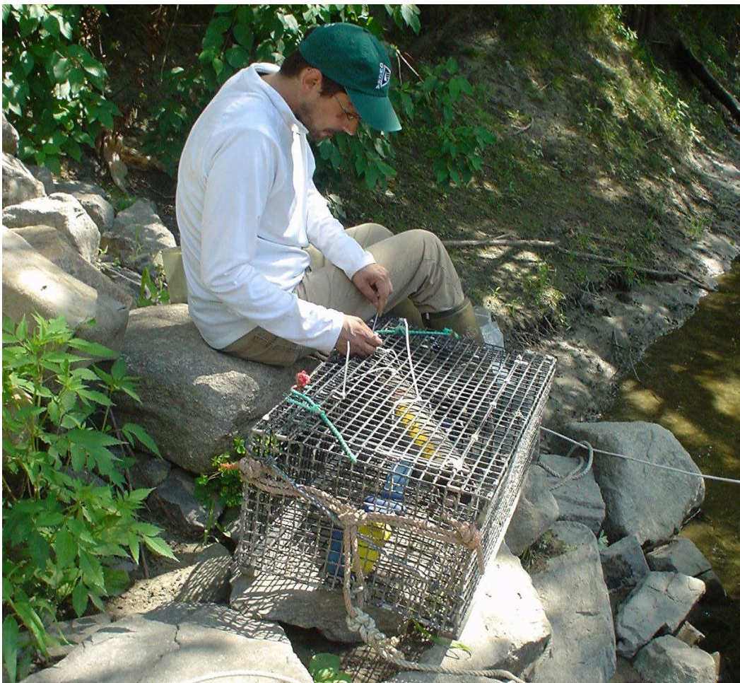
Figure 2: Datasonde deployment system being prepared by Cayce Dalton.
