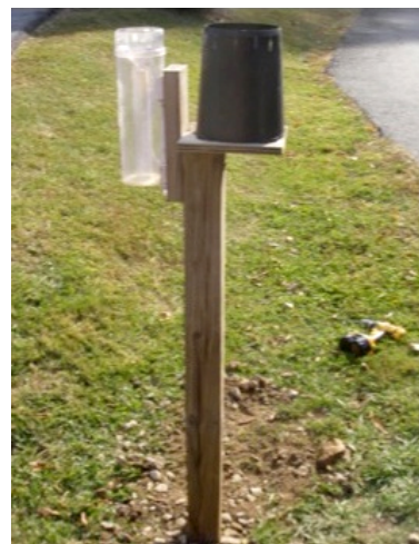
Figure C-16. Example of manual (left) and tipping bucket (right) rain gauges.
