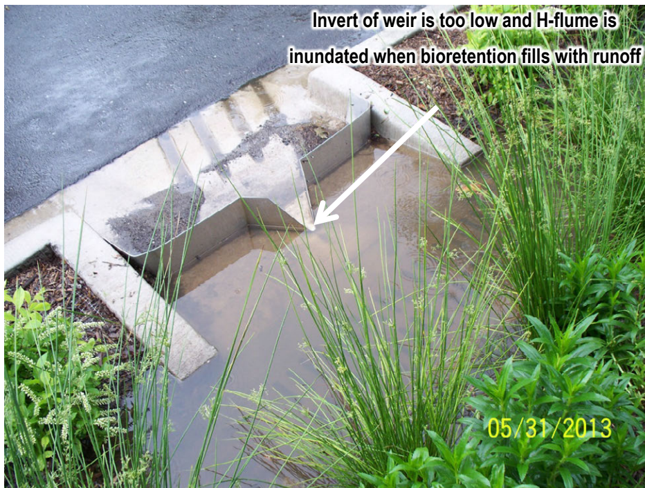
Figure C-14. Poorly installed H-flume at the inlet to a bioretention area in which the invert of the weir is too low, and tailwater from the bioretention will interfere with measurement.
