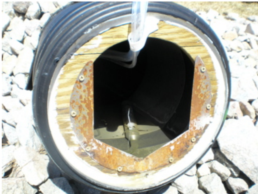
Figure C-9. Inflow pipe to bioretention area equipped with compound weir and bubbler for flow measurement. Water quality sampling tube and strainer are visible inside pipe.
