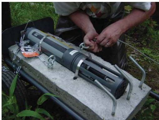
Figure 7-1. A YSI model 6600 data sonde being prepared for deployment using the 'tombstone' anchoring system devised by PRW.
