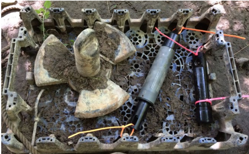
Site 1 Conductivity and Dissolved Oxygen Data Loggers
